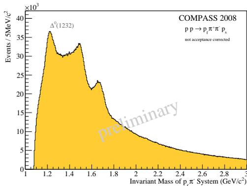
Figure 8: Invariant mass of the  $p\pi^-$  system with proton beam.
