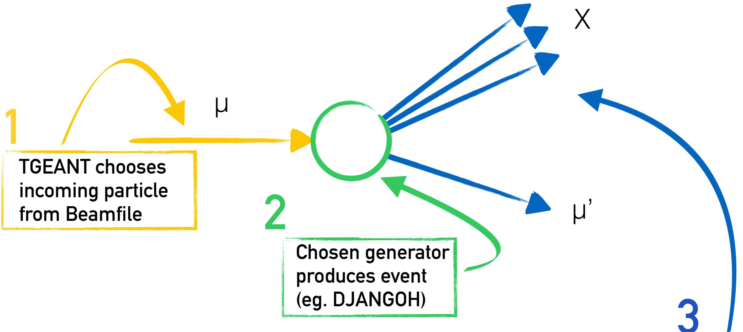
TGEANT recovers particles created by generator, kills incoming particles and creates outgoing particles
