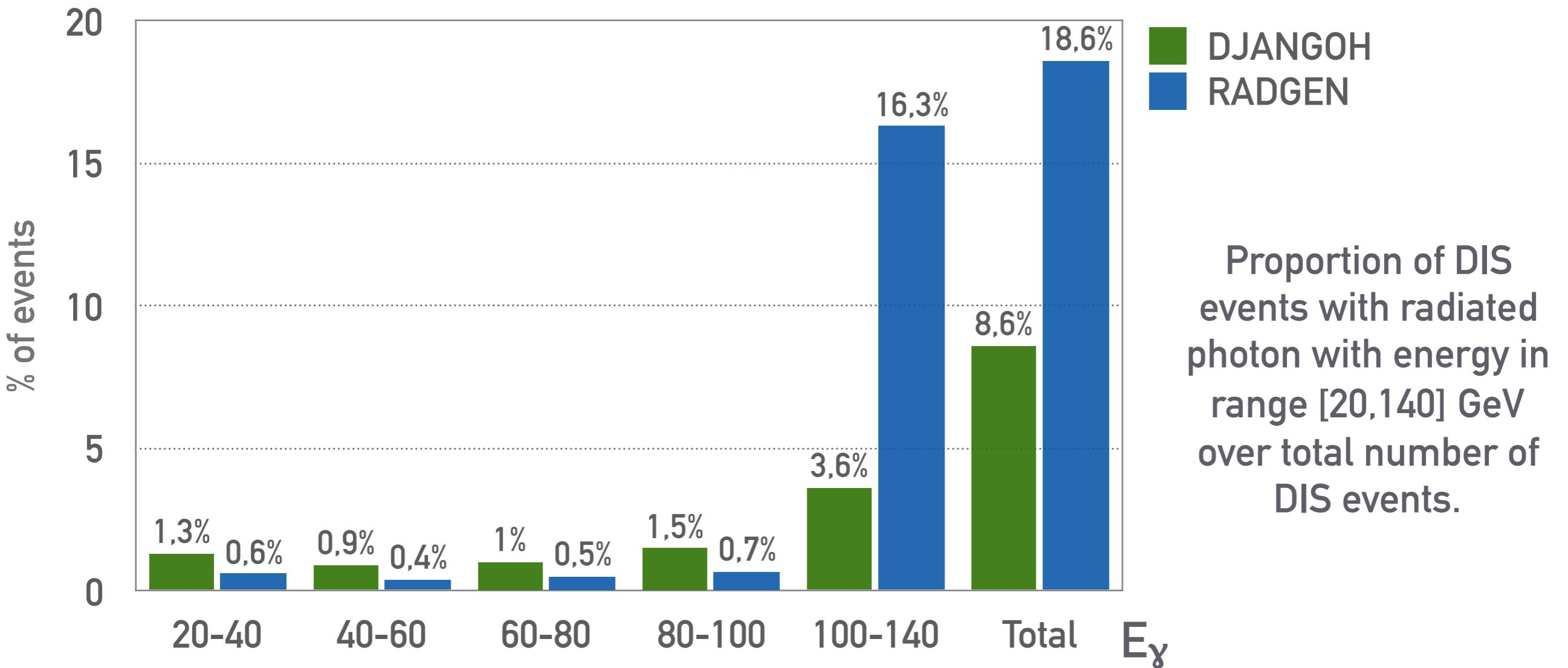
DJANGOH produces less hard photons than RADGEN
